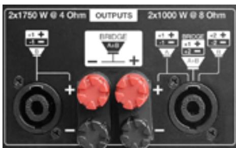
There are two speaker outputs: CH A and CH B both fitted with Speakon sockets and Terminal type (binding posts) connectors.
