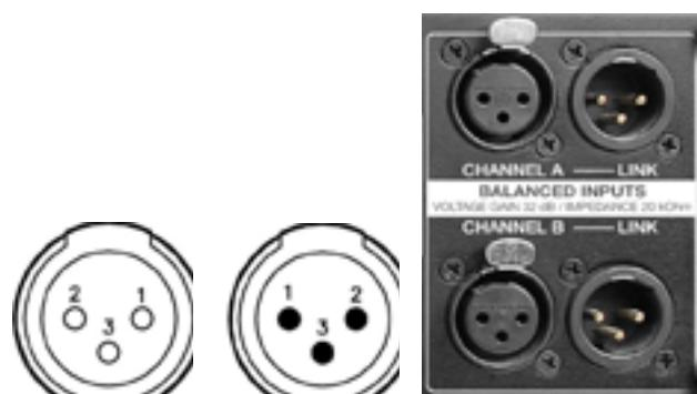
(\*) NOTE: This amplifier follows the ground interconnection specification defined by AES48-2005 standard of the Audio Engineering Society, on grounding and EMC practices for audio equipment containing active circuitry.
