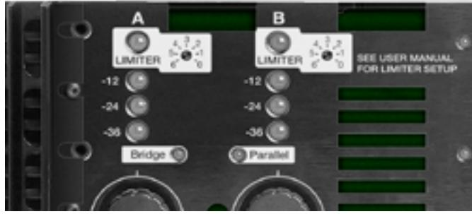
The factory setting for this parameter is set to fully clockwise, this way the device delivers its maximum power with minimum distortion thanks to its anti-clipping system.
