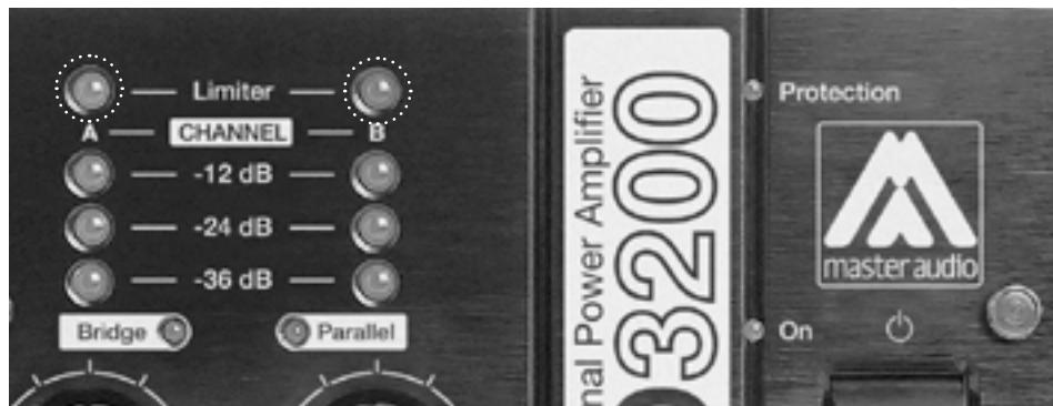
**! Make sure the LED LIMITER is not alight permanently !**
